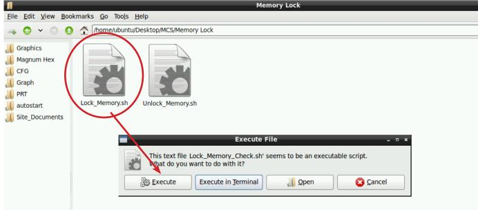
When the Lock Memory file is pressed it does an automatic reboot and autostarts MCS-Connect.
